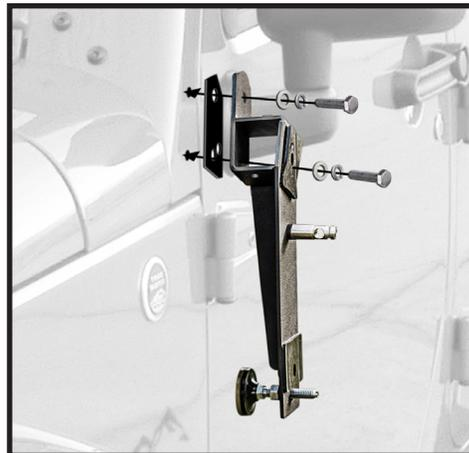
FIXEZ LE SUPPORT J-MOUNT SUR LA CHARNIÈRE DU PAREBRISSE AU MOYEN DES BOULONS, RONDELLES PLATES ET RONDELLES DE BLOCAGE FOURNIS ET BIEN SERRER COMPLÈTEMENT
