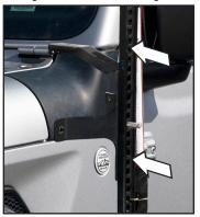
20. Attach Jack to Bracket assembly with Locking Pin extending through hole in Jack.
