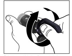
Fully insert vehicle key. Rotate clockwise while maintaining full key insertion until it stops *Avoid pulling up or down on key during coding.*
