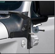
14. Place both Spacers (Gasket side against vehicle) into opening after removing bottom screws in Step 3.
