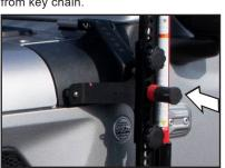
Push BOLT Lock securely onto Locking Pin.
