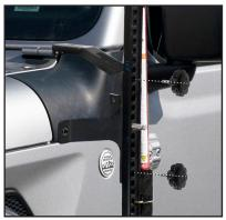
21. Install (2) Knobs through Jack and into threaded holes in Bracket. Use the threaded holes that line up best with the openings in the Jack you are using. (Hole spacing in the Jack varies by manufacturer).
