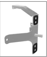
9. Attach Gaskets to top and bottom of Bracket assembly around threaded holes. Press firmly in place.
