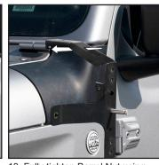
18. Fully tighten Barrel Nut using 8mm allen wrench.
