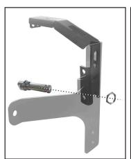
8. Insert Locking Pin through hole in Bracket assembly. Thread Panel Nut onto Locking Pin and tighten.
