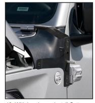
19. With hood open install Cotter Pin through hole in Security Screw.
