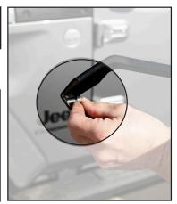
12. Insert Barrel Nut in Brace hole closest to the windshield.
