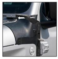
13. Thread Barrel Nut onto window hinge. Using 8mm allen wrench turn it onto the post a few turns but do not tighten fully.
