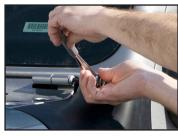
11. Using a T45 Torx remove Hinge nut from window Hinge.
