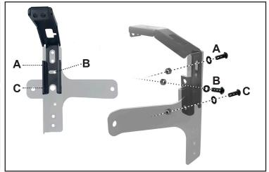
7. Attach Brace to Jack-Mount Bracket using (3) 20mm Screws, (3) Flat Washers and (3) Nuts. Line up image as shown.
